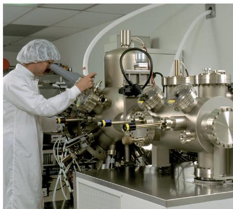
**Catalysts are substances that allow chemical reactions to proceed at lower temperatures. Even though, many chemical reactions that involve catalysts still occur under extreme conditions. For example, Fischer-Tropsch reactions, where a gaseous mixture of carbon monoxide and hydrogen is converted into (liquid) hydrocarbons at high temperature and pressure over a solid catalyst.**
